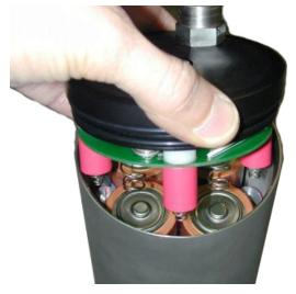
Figure 3. Correct end cap position for installation
