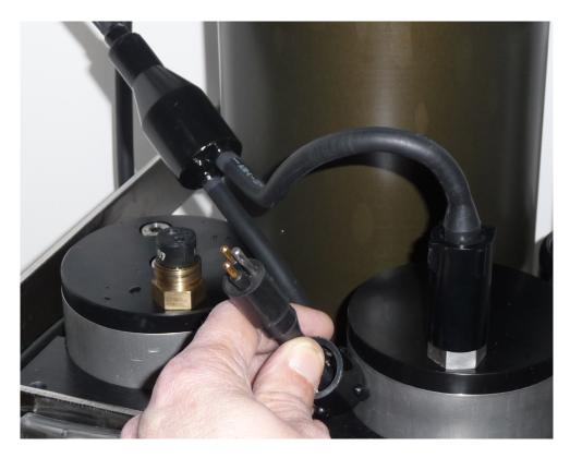
Figure 4. Beware: when one leg of the Y is plugged into a pack, the second plug is live.
