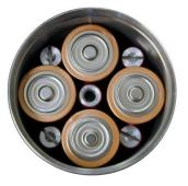
Figure 2. Cell orientation
